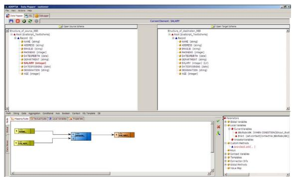
Create a link from the output of the custom method node to the input of the target element (see Figure 406).
