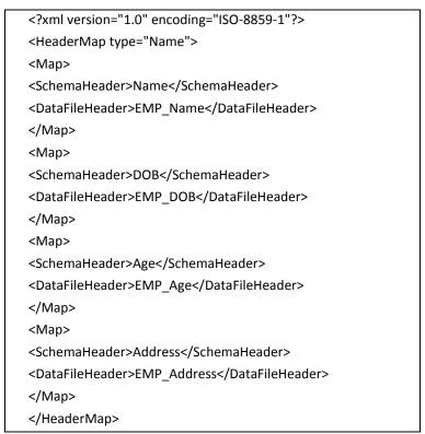
Figure 212: XML to map Field Name with Data Header
