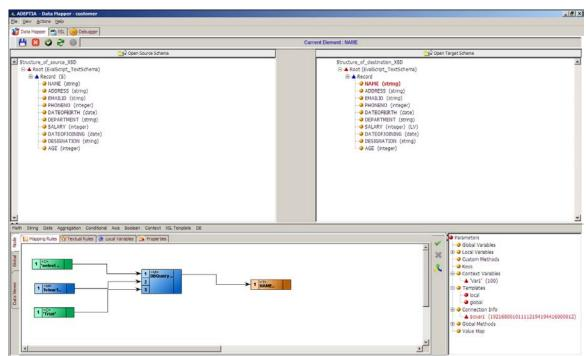
11. Create a link from the output of the DBQuery node to the input of the target element (see Figure 381).
