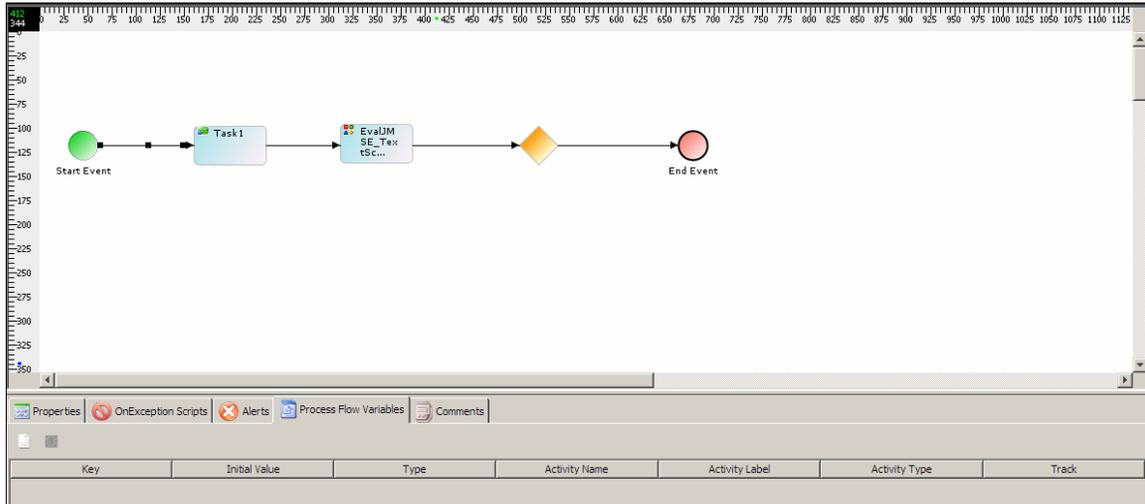
Figure 16.34: Process Flow Variable Panel
